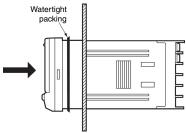
3. Insert the fixture into the grooves on the left and right sides of the rear case and push until it reaches the panel and is fixed in place.
